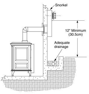
Figure 22 - Snorkel Termination with Drainage Pipe
